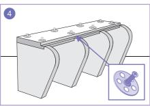
4. Screw and washer fix through the Seat Top into each Profile at the rate of two fixings per Profile. Check for square and allow to cure for a few minutes.
