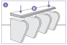
**3.** Take the Seat Top **(Part B)** and press it firmly into place in the recesses.
