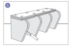
**5.** Apply a generous bead of adhesive to the front, curved edges of each profile and to the notched parts of the Seat Top.
