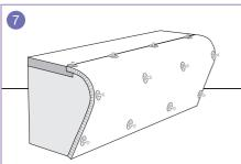
7. Screw and washer fix through the Flexo Plus Seat Front into the curved edges of each profile at the rate of three fixings per profile. Position the first fixing where the Flexo Plus inserts into the notched edge of the seat top, the second on the front curve and the third near the base.
