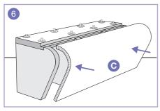
6. Now position the Flexo Plus Seat Front (Part C) firmly against the adhesive beads making sure that the cuts are facing inwards. Any overlap at the base can be trimmed later.
